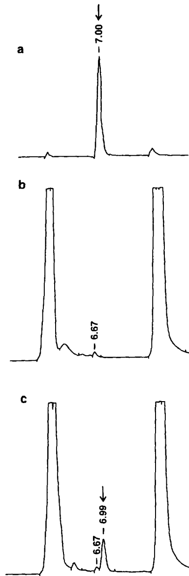
Fig. 3. HPLC analysis of the product. Authentic LacNAc was separated and the retention time was determined to be 7 min (a). The reaction mixtures using either lysate of BT/pDP34 (b) or BT/pDPsGT (c) was separated on HPLC. The position of LacNAc is indicated by the arrow. Note: the peaks showing a retention time of 6.67 do not correspond to the authentic LacNAc profile.
